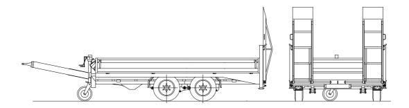
**Axles:** Fast-running axles type Knott with S-cam brakes, leaf spring and weight adjustment
