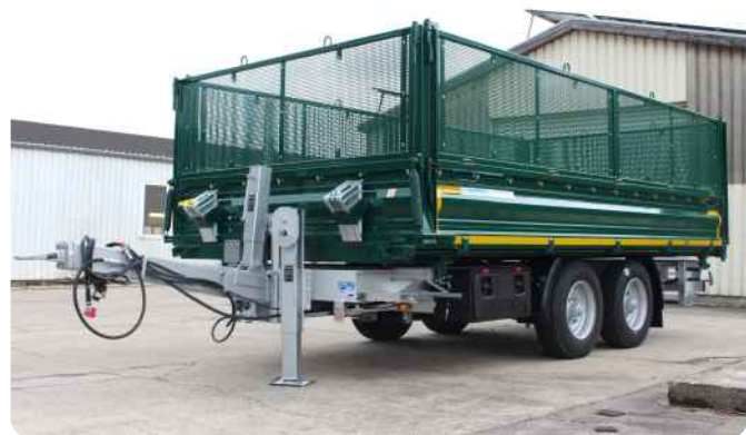
Leaf extension, 70cm high, made of punched perforated plates, attachable, swinging to the side and rear. With reinforcements and eyelets for attaching and detaching the additional drop sides.
