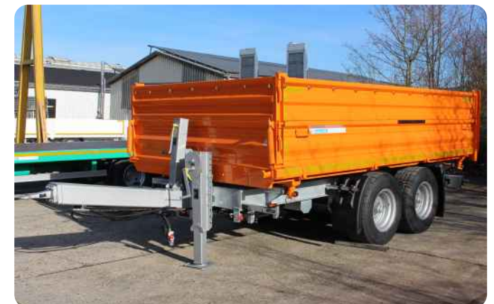
Additional steel drop sides, 400 mm high, all round; fixed at the front, swinging at the sides and rear; with net hooks and spring lifters
