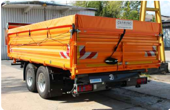
Rear wall as two-part hinged door instead of swing flap, doors can be hung from the side, opening radius on each side approx. 1.20m; with additional steel drop sides, wide tyres and TELL One roll-off tarpaulin
