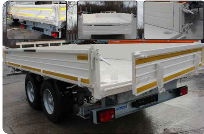
Rear wall as one-piece hinged door swings and folds down; opening radius approx. 2,40m
