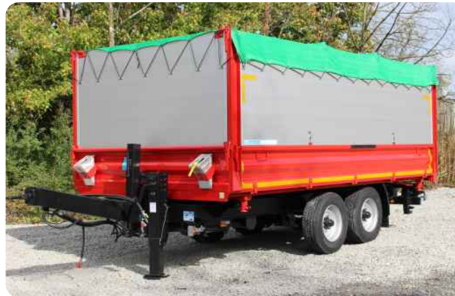
Chopper body 120cm high, made of anodised aluminium profiles, attachable, swinging to the side and rear. Removable front and rear drop sides; with eyelets on the side walls for hooking and unhooking.
