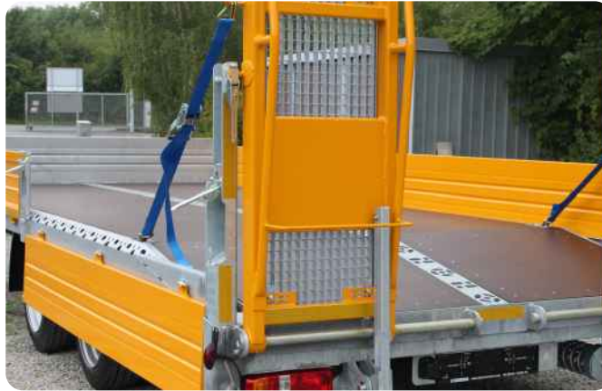
Flexible load securing with the center VarioO lashing rail for various sling equipment and the outer profile with double perforation "VarioFrame"
