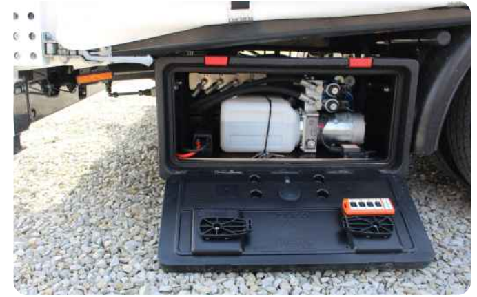
24-volt compact electro-hydraulic power unit with 2200W power for operating the hydraulic ramp jacks, incl. radio remote control! Installed in a plastic tool box on the passenger side of the low loader, 2-pin NATO socket attached to the front wall, supply line to the pump.
