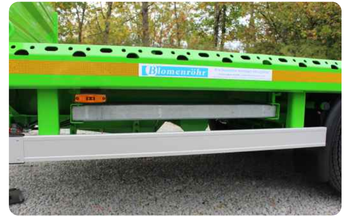
Stake holder under the loading area with locking mechanism, VarioFrame outer profile
