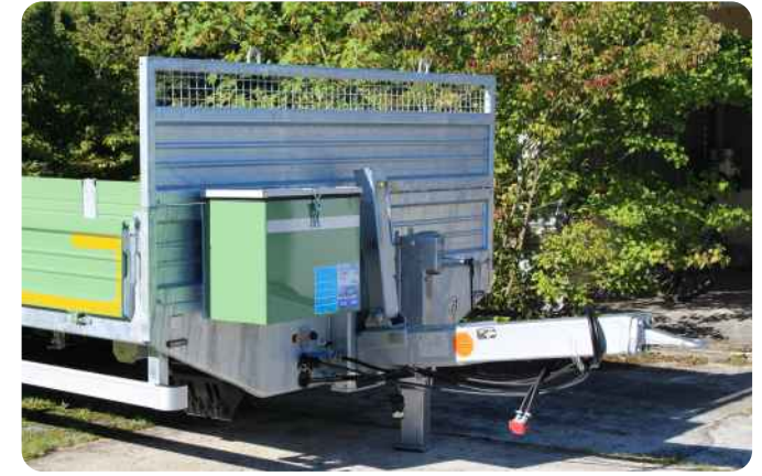
Front wall raised from steel drop side, with additional frame extension; self-made steel tool box with aluminum cover
