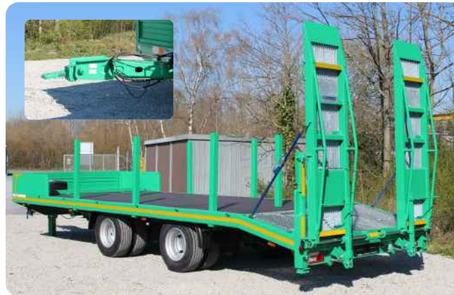
Grid gratings in the ramps and access slope, stanchions on the side of the loading area, retractable lashing rings, swivel eye 40/50 mm
