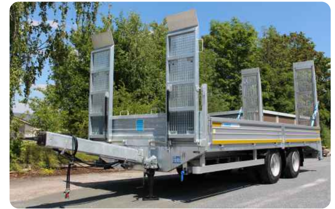
Ramps with 3.5t load capacity, for driving onto the towing vehicle, with gas pressure shock absorbers, movable. Only possible with fixed or hydraulically height-adjustable tow bar
