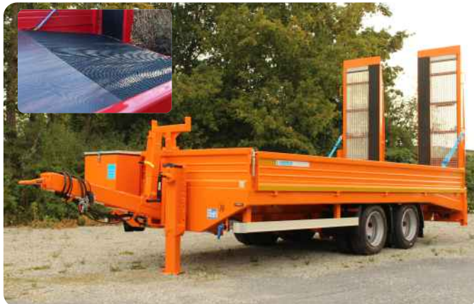
On 80cm widened ramps with HEGE rubber covering in the middle; telescopic storage for the milling conveyor at the front, HEGE covering also possible in the ramp!
