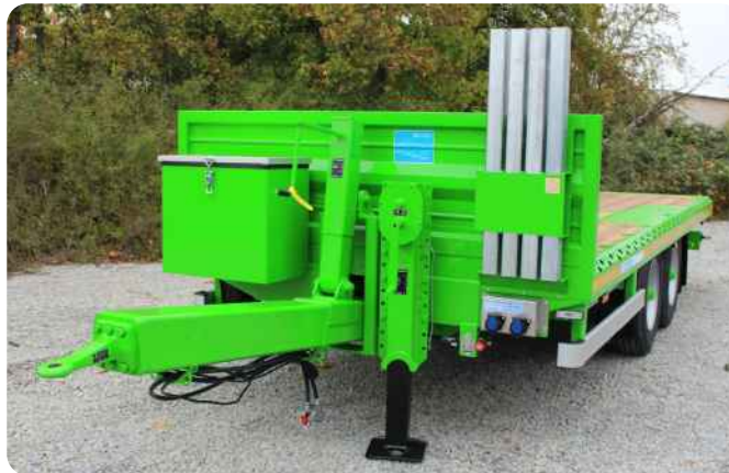
VarioSave stanchions (available in different lengths) with stanchion magazine on the bulkhead, steel tool box from our own production with aluminum cover
