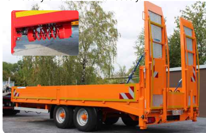
Operate widened and extended ramps with spring lift mechanism, fully collapsible, aluminum drop sides split down the center, with reflective marking
