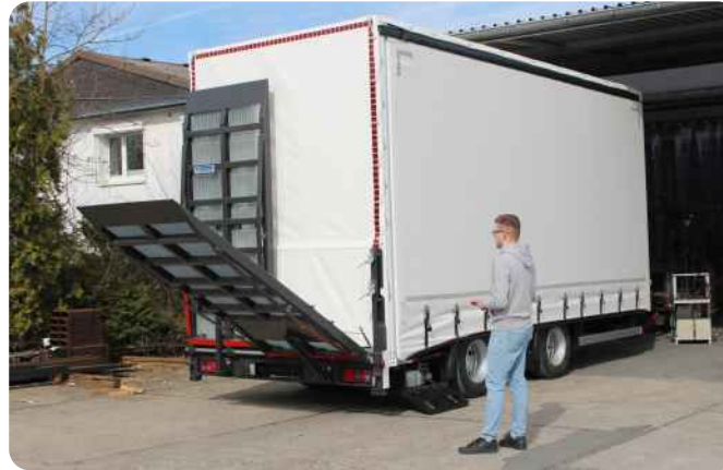
Hydraulic ramp jacks in combination with an electro-hydraulic compact power unit: double-acting cylinders with check valves are mounted in a protected position under the loading area and connected to the electro-hydraulic pump. The cylinders are operated via the radio remote control. The ramps can be controlled individually or both simultaneously.
