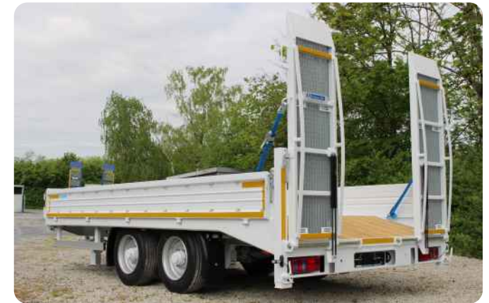
Double gas struts as lifting aids
