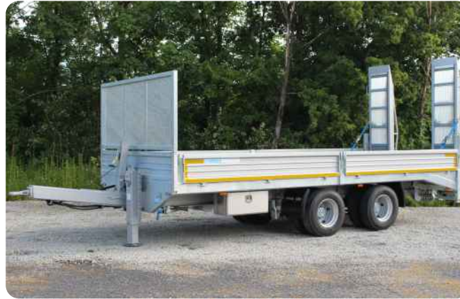
Front wall made of perforated plate, pluggable or fixed; stainless steel tool box attached to the side, divided side panels
