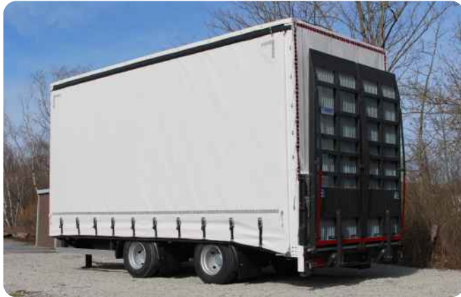
Closed tail lift with gratings, divided in the middle, tarpaulin cover frame with sliding tarpaulin, interior lighting and rear roller tarpaulin
